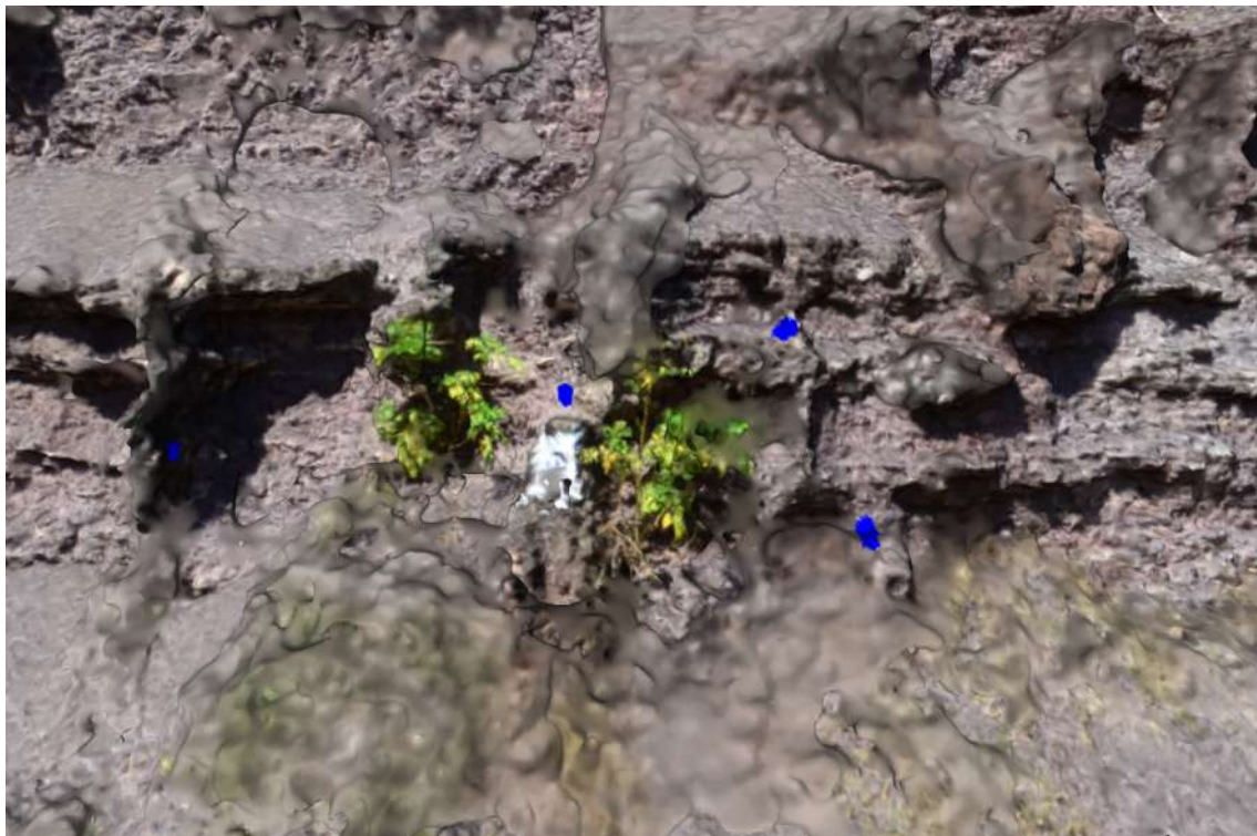
Figure S2. Example of distortion and artifacts generated on the DOM. The surface sampling was not performed on these areas as the surface distortion would significantly affect measurements.
