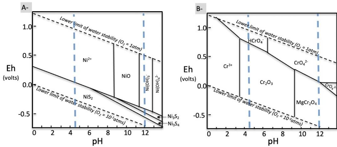
Figure Suppl: Simplified Pourbaix diagram for nickel (A-) and chromium (B-) species dominating in diluted aqueous solutions, at 25°C and 1,013 bars. The broken vertical lines represent the normal pH range in natural waters
